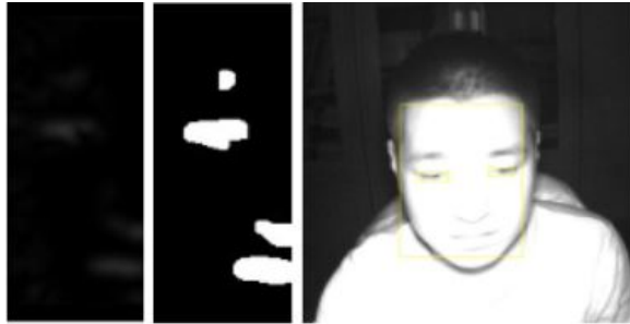
Fig. 5. The Accurate Positioning of eye
